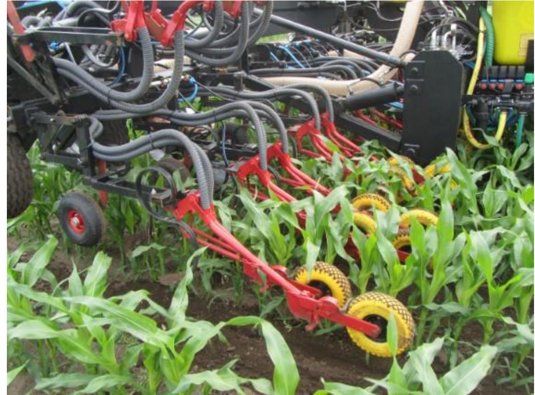
Specific machine stations are developing equipment for sowing grass in maize using pressure from the wheel. Photo: Henning Sjørsløv Lyngvig, SEGES.
